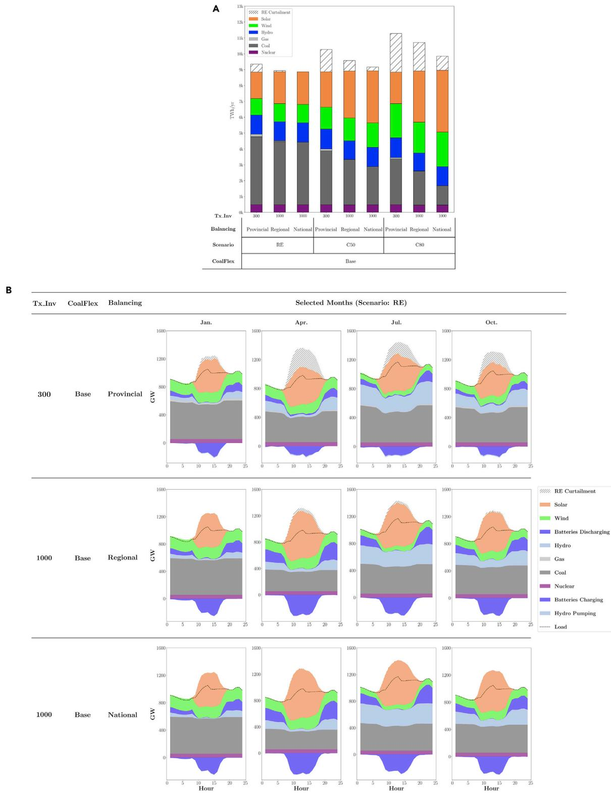
**Figure 5. China national annual generation and average dispatch with two transmission cost settings under different balancing strategies**
