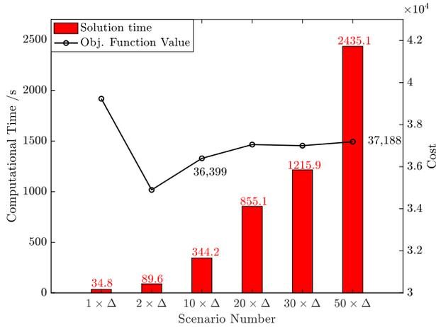
Fig. 4. Sensitivity analysis on the scenario number.
