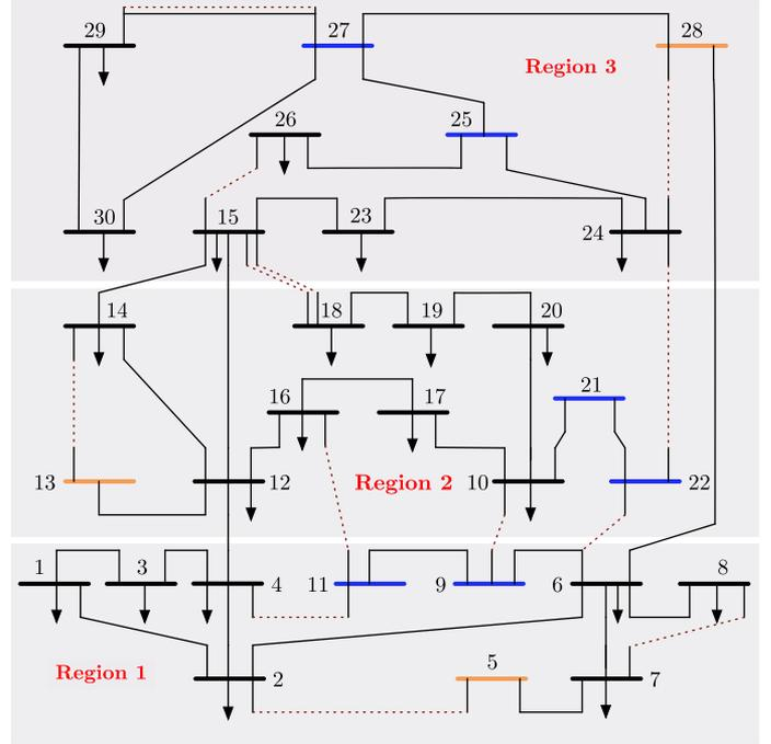
Fig. 3. System topology of the modified IEEE 30-bus system.
